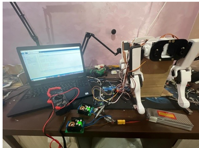
Figure 5. Arduino Uno microcontroller setup with connected servo and sensor interfaces
