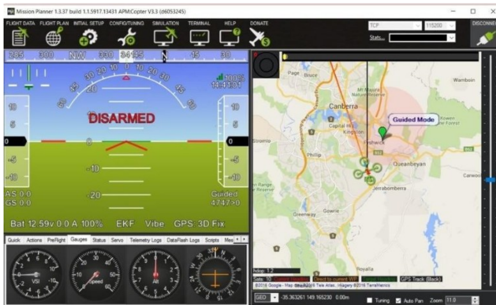
Figure 2. Ground Control Station (GCS) Mission Planner Application
