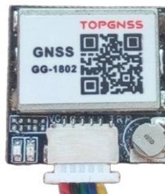
Figure 5. Global Positioning System (GPS) GNSS GG-1802
