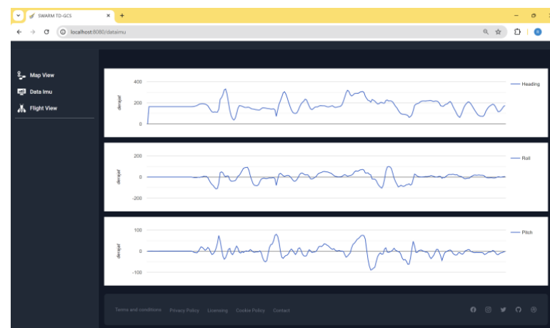
Figure 15. Inertial Measurement Unit (IMU) Data Menu Display
