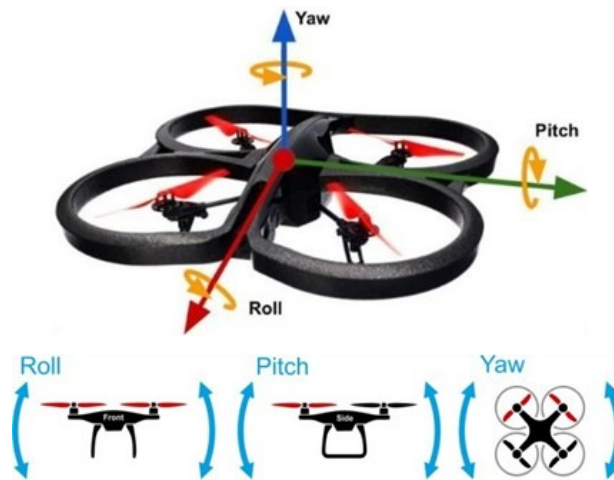
Figure 10. Three axes of rotation on an Unmanned Aerial Vehicle (UAV)
