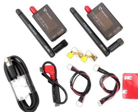
Figure 7. A pair of 3D Robotics (3DR) 433 MHz Radio Telemetry Modules
