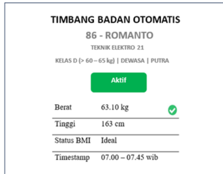
Figure 4. HMI display of the scales
