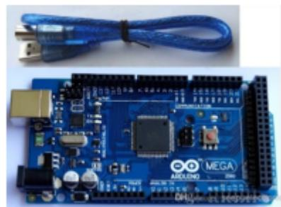
Gambar 5. Arduino Mega2560
