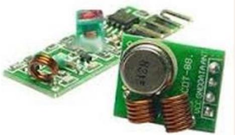
Gambar 3. RF Module Board 433 MHz
